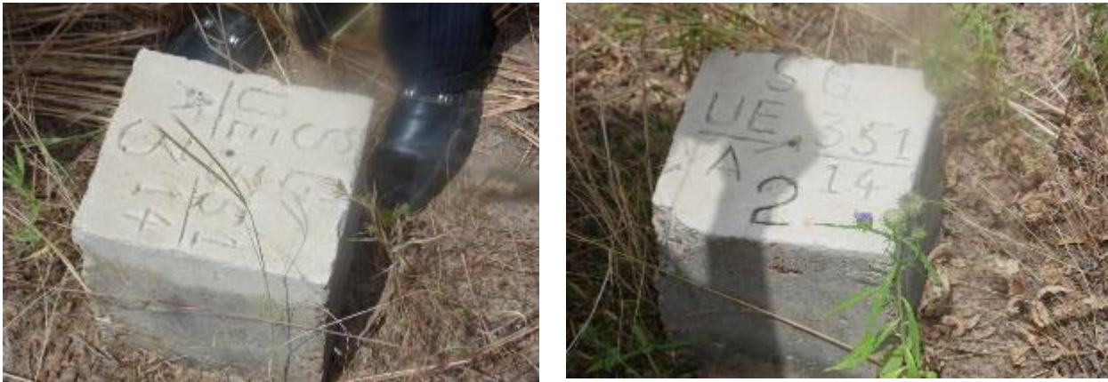
Plate 3-1: Survey Pillars at Solar Power Project Site at Asegba
